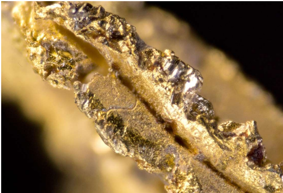
Detail of one of the studied samples: Gold with goethite and hematite.
