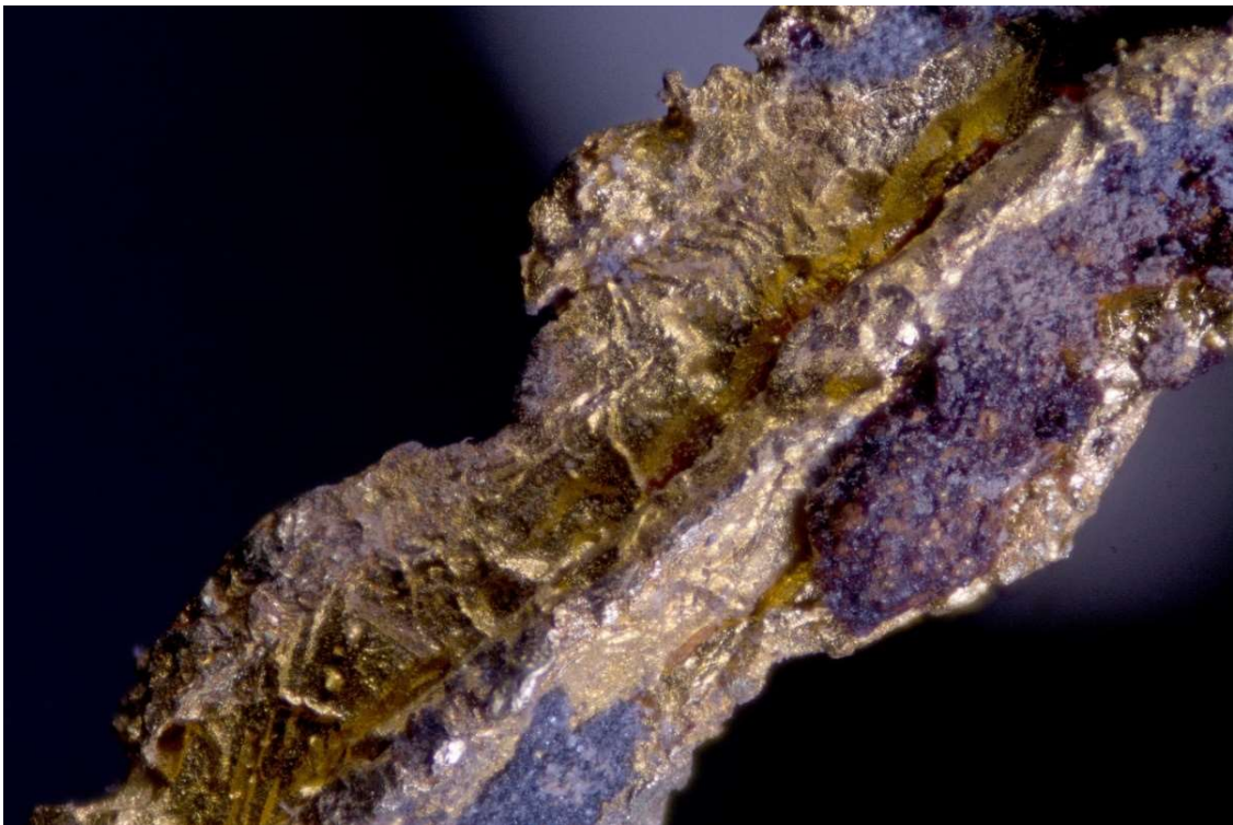
Goethite and hematite on gold. Iron oxides do not appear usually mixed, rather are forming differenced zones.
